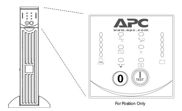
The ON and OFF buttons power the UPS and act as master controls for the connected equipment if connected equipment is switched on. The UPS remains on as long as it is attached to utility power and the switch is not pressed.
